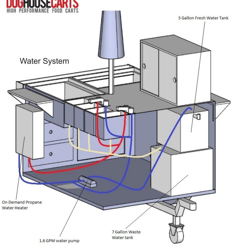
Blue Line: Cold Water Red Line Hot Water White Line: Waste Water
